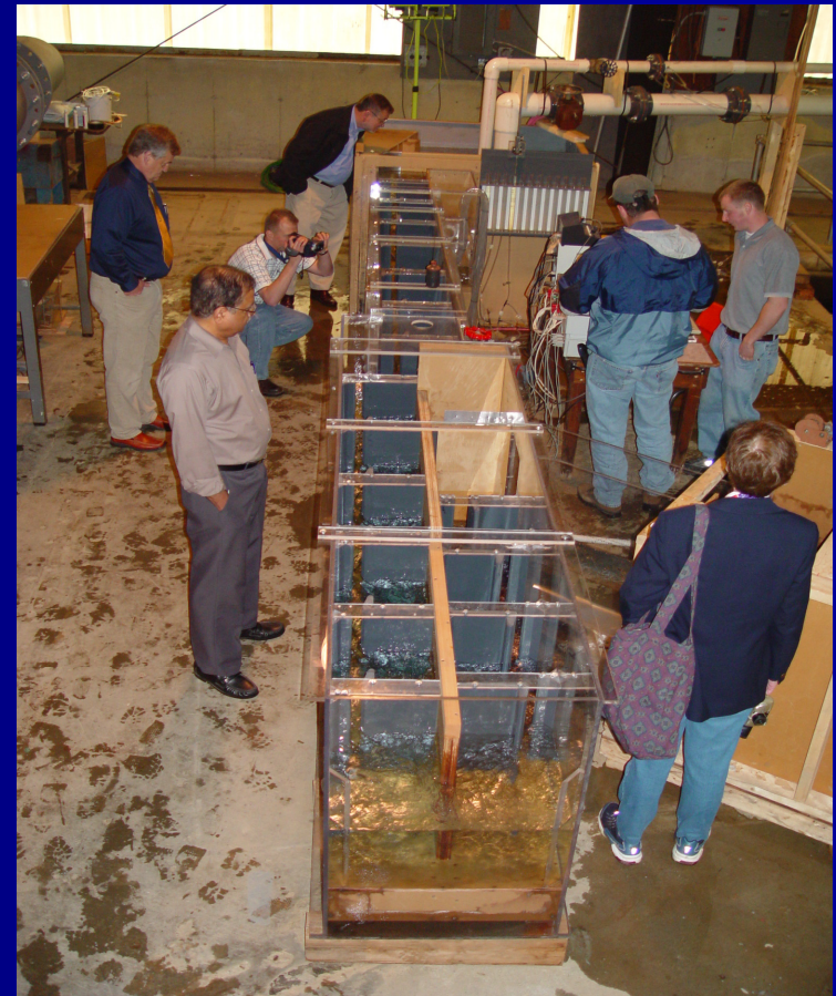
9:1 scale of the Fairmount Fish Ladder (Alden Laboratories, Worcester, MA)
