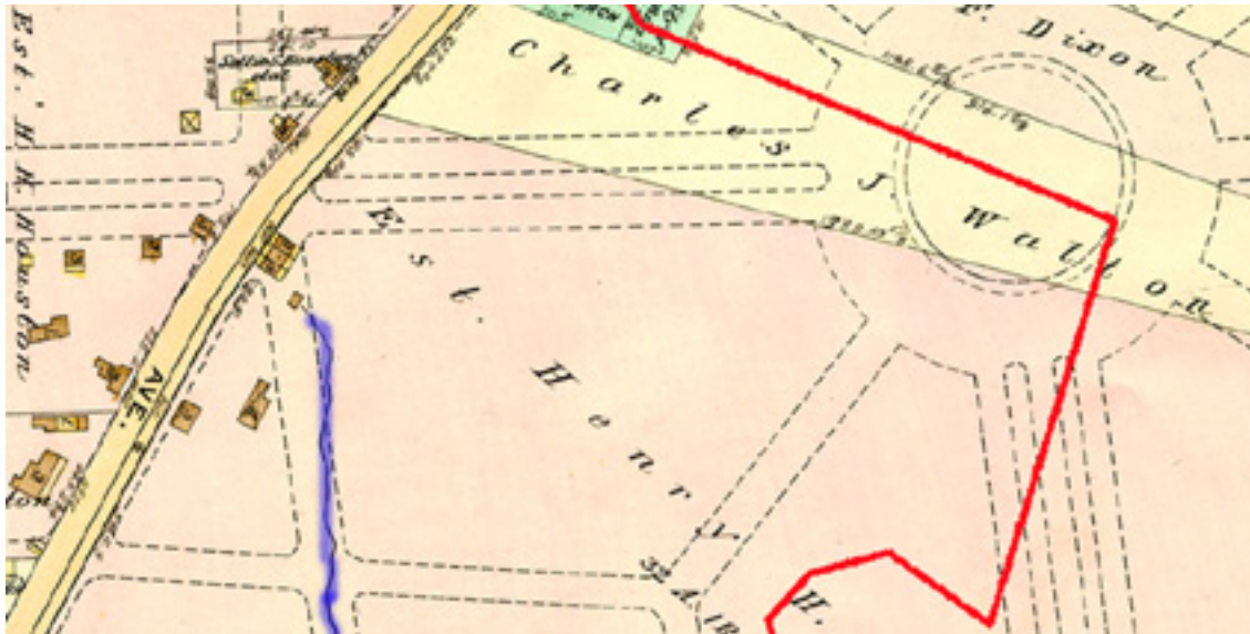
Red line indicates watershed boundary; street on left is Ridge Avenue; blue line is stream, ending at spring house
