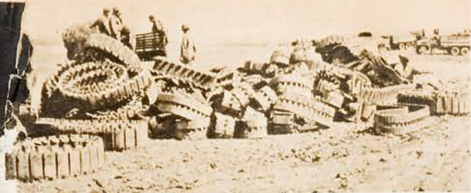
Treads from the battlefield are piled in huge heaps behind the lines to await repair. These serve as replacement parts, to be used on tanks or half-track vehicles whose treads have been battle-damaged beyond hope of recovery.
