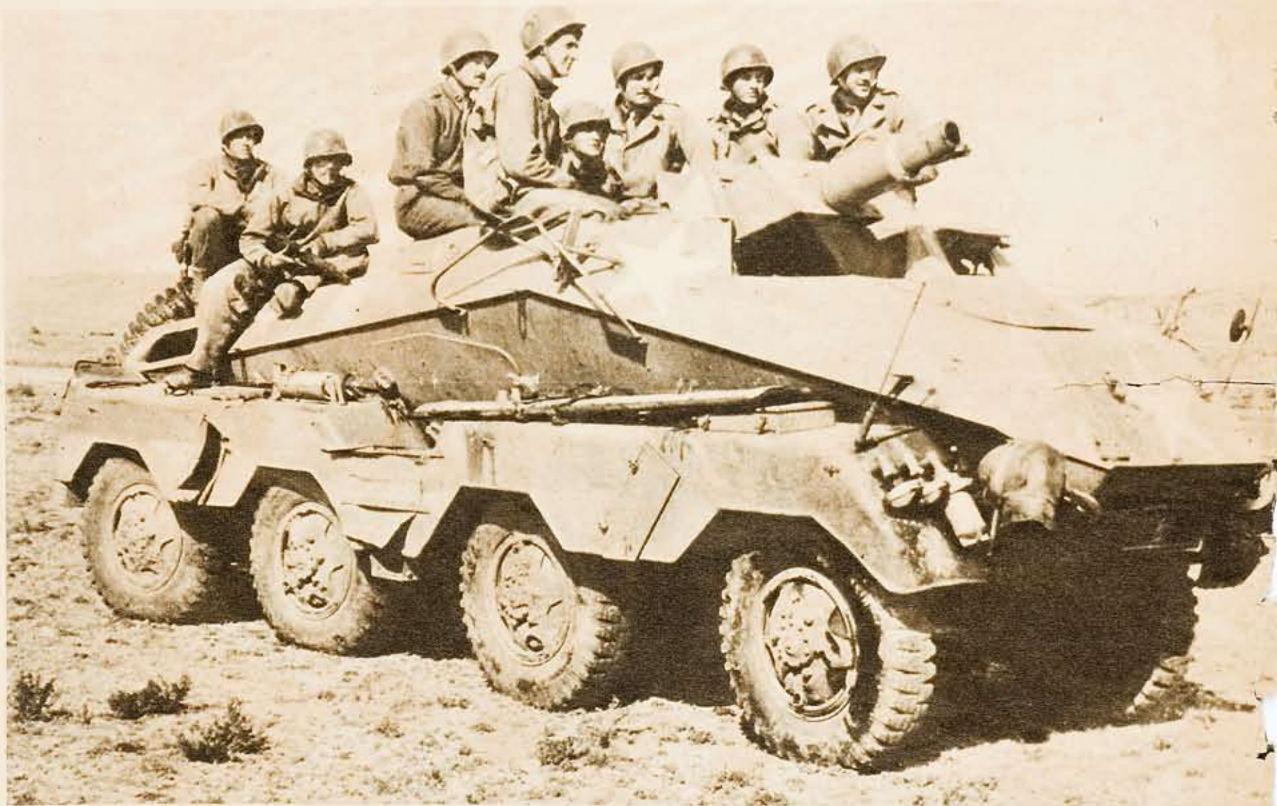
Prize piece of salvage is a German tank destroyer, now in use by the U. S. Army. It is armed with a howitzer, has dual controls for operation forward or backward.
