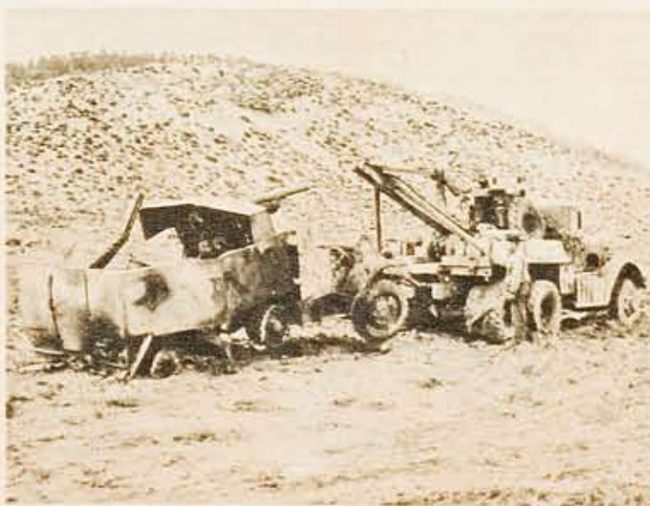
Badly battered, but still considered worthy of salvage, a half-track mounting a 75-mm. gun is dragged from the battlefield. Parts which are too damaged for further use are tossed on a scrap pile and eventually sent to steel mills.
