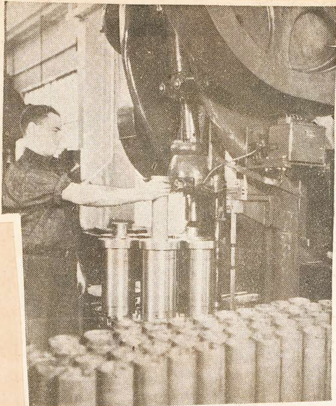
This press tapers medium calibre cartridge cases, prepares them for next step in assembly line
