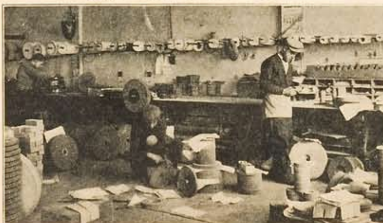
FIG. 7 — Inspection Department, where Wheels are micrometered and checked carefully for all dimensions and composition.
