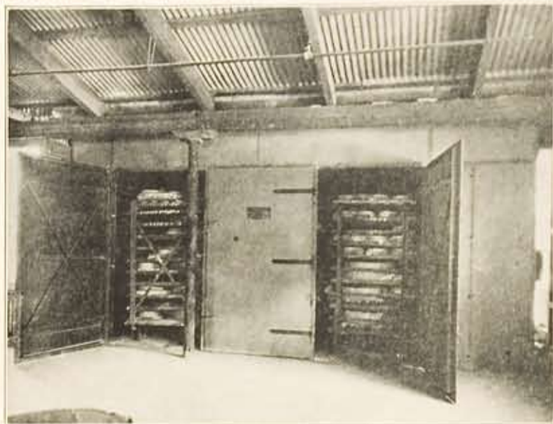
FIG. 2 — Humidity Dryers, showing racks of Grinding Wheels
