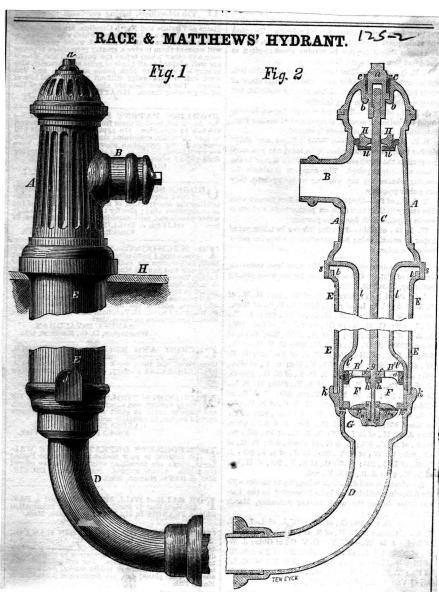
The chief features of novelty in this hydrant are that, by the peculiar arrangement of the valve, the waste pipe is opened as the induction pipe is closed, and it can be readily removed from its base without the necessity of excavating.
