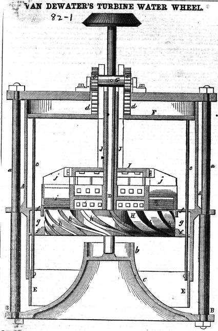
The accompanying engraving is a vertical | to cross bars, F. to which vertical racks, ddsection of the water wheel of Henry Van Dewater, of the city of Albany, N.Y., embracing an improvement on his patent of October 1853, for which he has just taken measures to secure a patent.
