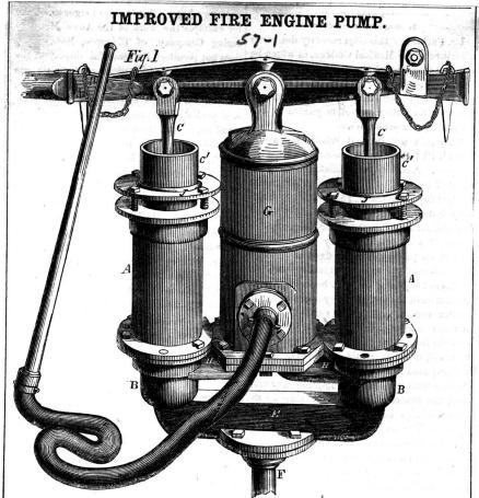
The annexed engravings illustrate a very suitable term, for each valve is composed of excellent improvement in pumps, by Mr. two spheres, viz.: a central metallic sphere Ambrose Tower, of this city, who has made application for a patent.
