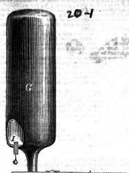
The annexed engraving is a side elevation partly in section of an improvement in water closets, for which one patent was granted to F-H. Bartholomew, of this city, in 1846, and an other on the 14th of last February, (1854).-The engraving represents a double valve arrangement.
